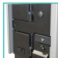
Kotlovska vrata, termomanometer, regulator propuha
